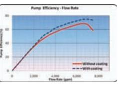
**Figure 1.** Pump efficiency evolution as a function of flow rate as calculated from data collected in November 2006 and March 2007.
